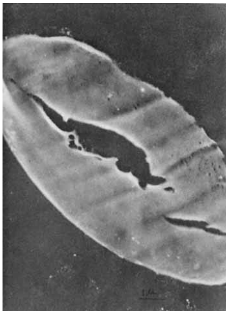
Fig. 8. Electron micrograph of expansion patterns of cross section of form D cotton, treated with NaOH and then crosslinked with formaldehyde. \text{CH}_2\text{O} , 2.85%, crosslinks, 0.1540/GPU; G = 0.93 .
